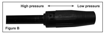
2. Do not dilute the detergent. The detergent sprays out at low pressure only. Slide the Spray Nozzle out for low pressure. The pressure washer will draw the detergent up through the Detergent Suction Hose and mix the water and detergent automatically, at about a 6% detergent 94% water ratio. **See Figure B.**
